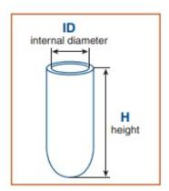
\* Extraction thimbles in accordance with DIN 12449 for extractors with defined nominal volumes according to DIN 12602 and 12604
