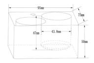
Block with 2 holes for 50 ml flat bottom tubes for thermoblock with settable temperature from 25 to 200 ° C
